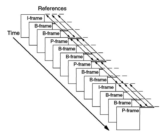
Figure 19. Typical MEPG-2 Picture Sequence Showing Picture Types
